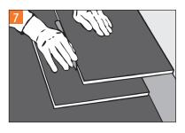
7 Fitting the last row of planks: Place the plank to be repeated exactly on the last installed row of planks. Then mark the longitudinal section using another plank. This type of marking leaves sufficient distance to the wall in order to angle the last row by means of pull bar.
